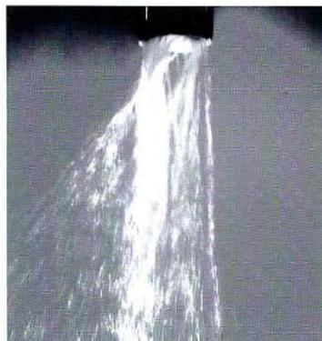
Lime builds up fast on wire mesh screens and blocks off the water and air passage. The stream loses aeration and starts splashing and the flow rate decreases.
