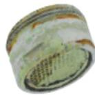
Lime build-up on wire mesh aerator screens dramatically shortens the life of aerators. Dissolved lime, naturally found in drinking water, builds up on wire mesh screens and slowly closes the air inlets.
